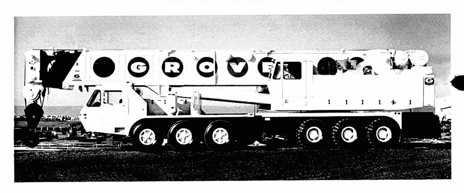
THE GROVE CARRIER The Grove designed diesel powered carrier is manufactured by Grove to match the particular requirements of the TM1275 crane and it's long boom capability. The all-welded box-beam design steel frame in combination with five point outrigger configuration provides a stable lifting base for 360° lifting capability. The two man acoustically treated cab can be equipped with air conditioning.
